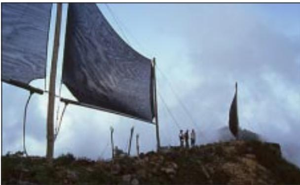
Fig. 3 : Fog collector with anemometer to detect the wind direction
