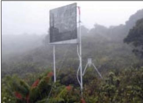
Fig. 2 : A fog harvester arranged in perpendicular direction of wind can condense fog into water
