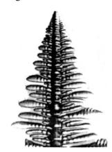
**Fig. 1.** *Microstructure of SCN*  $\times$  50.
