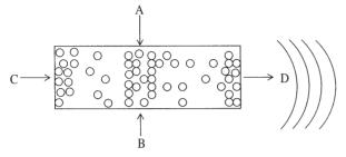
Fig. 2 : SASER (A. suspended tiny bubbles of gas, B. set of bubbles runging, C. pass sound waves & D. sound waves emerge)
