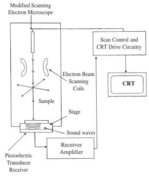
Fig. 1: Scanning Eelctron Acoustic Microscope
