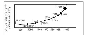
PM: Preventive Maintenance: CMMS: Computerised Maintenance Management System; RCM: Reliability Centred Maintenance: TPM: Total Productive Maintenance: PDM: Predictive Maintenance: PAM: Pro-Active Maintenance. RBM: Reliability Based Maintenance
