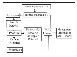
Fig. 2 : Cycle chart for condition based monitoring system
