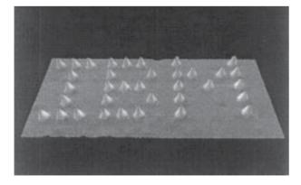
*Figure 1.* IBM's Initials spelled with nexon atoms (Courtesy : IBM Research, Almaden Research Centre) The image now hangs in the IBM's "STM" gallery (http://www.almaden.ibm.com/vis.stm/atomo.html).
