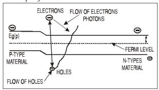
Fig. 4. P-N-Junction Electric Fields Photons incident upon n-type material surface ionitiates ther charge separation process.
