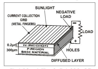
Fig. 1. Schematic View of a Typical Solar Cell
