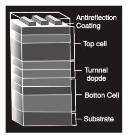
Fig. 3. Multi-Junction Photovoltaic Cell
