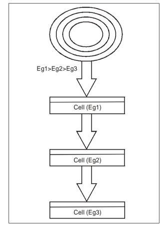
Fig. 2. Working Principle of a Solar Cell
