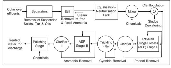
Fig. 1 : Process flow diagram for coke oven effluent treatment
