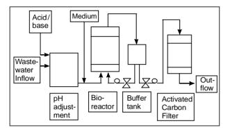
Fig. 1 : A schematic diagram of a mercury removal plant using a bioreactor
