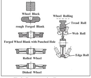
Fig.2. Forging and rolling sequence
