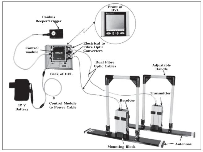
Fig. 2 : The complete low frequency pulse EKKO PRO hand held Assembly
